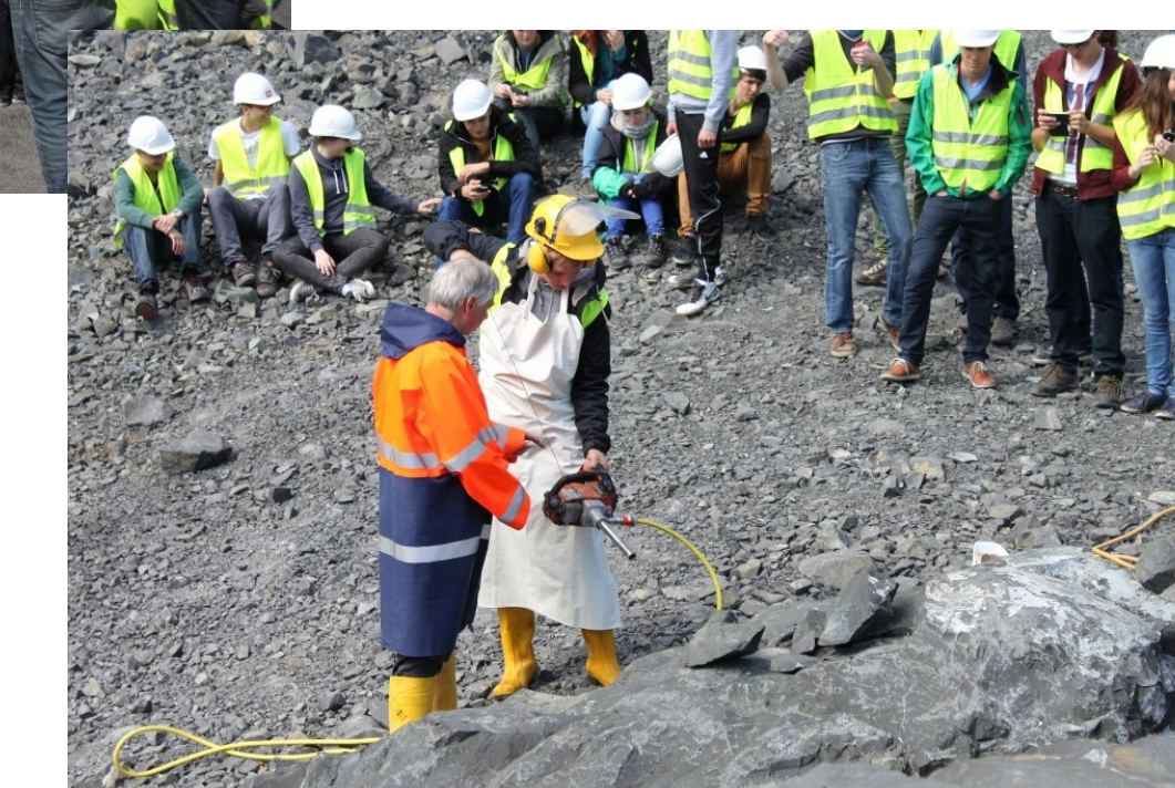
Fig. 9: (Below) Franz Pusterwallner (Montanuniversität Leoben) demonstrates use of the drill machine to a student from Graz. The machine is used to take cylindrical samples from rock.
