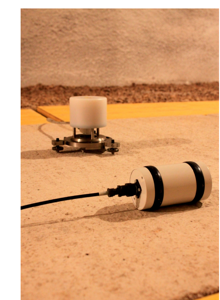
Fig. 2: Two of the stations use a scalar magnetometer (front) for measuring the total field strength and a variometer (behind), which determines the three-component variations in magnetic field orientation.
